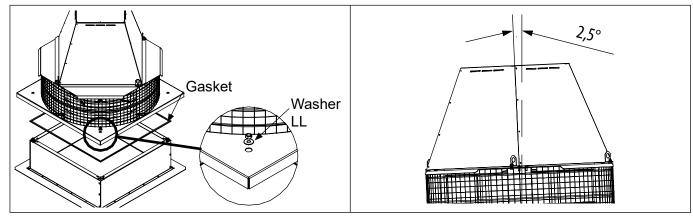
The base of the roof fan must completely cover the up-stand to ensure a good seal. Ensure that the support is adapted to the weight of the fan and its accessories. Fit the fan by means of the 4 holes Ø20 provided for this purpose. It is recommended to use LL washer. Improper tightening of the fixing screws may cause noise and vibrations. Once the fan is properly fitted, make sure the motor impeller rotates freely without friction or noise.
