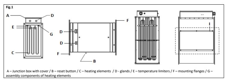
To gain access to the inside of the machine, please disconnect the power, then unscrew the screws and remove the cover. The cover
