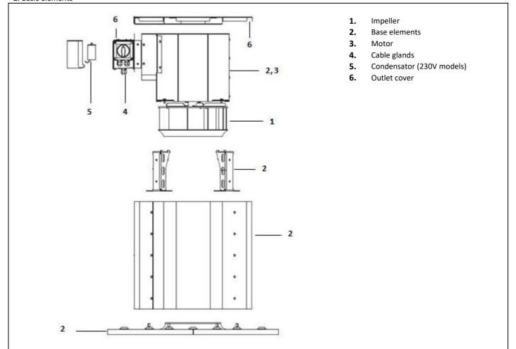
Base elements (2, 6) made of galvanized steel sheet or aluminium. Impeller (1) made of painted steel, galvanized steel sheet and steel and aluminium elements. Fasteners made of aluminium, steel, galvanized steel and stainless steel have been. The fan has been sealed with PTFE sealings and silicon. Additionally, the base has been sound-proofed with insulation mat.
